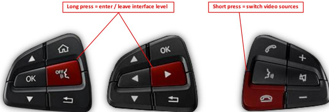
**Long press “handsfree mode OFF”** respectively **long press “right arrow”** button to choose the interface as current video source.
