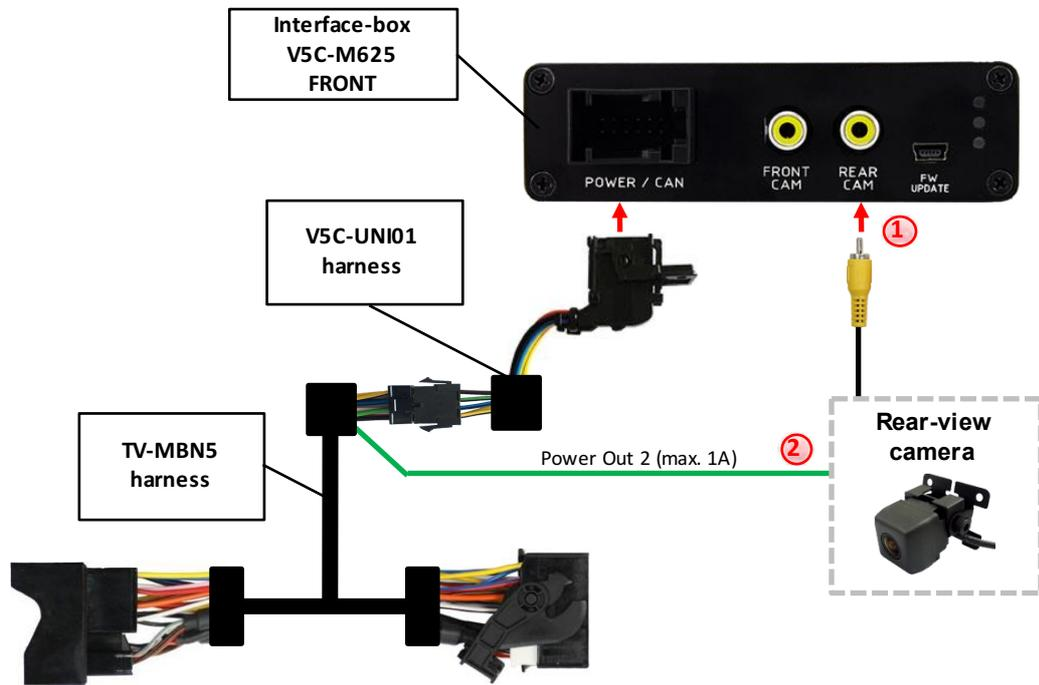
① Connect the video RCA of the after-market rear-view camera to the female RCA connector "REAR CAM" of the interface box V5C-M625.
