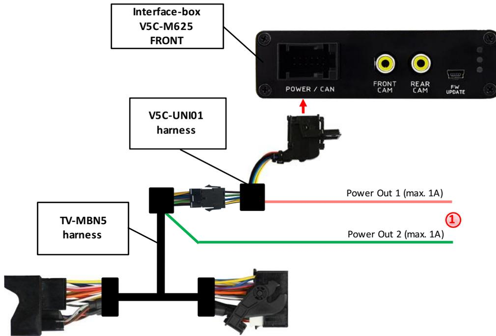
① You can configure the both +12V trigger outputs separately. The pink wire is POWER OUT 1 and the green wire is POWER OUT 2.
