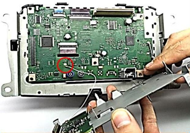
**4** Carefully separate the metal cover and disconnect the small Coaxial wire connected in between.
