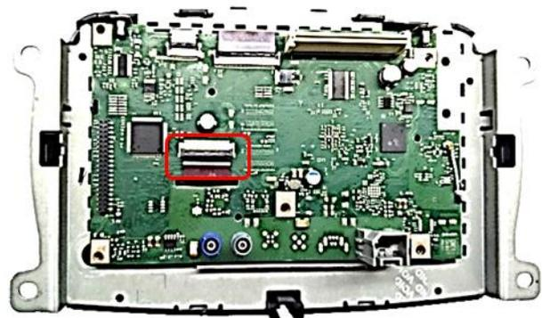
**5** Disconnect the ribbon cable from the mainboard's ribbon cable base, as shown above.
