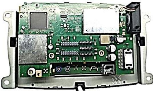
**2** Carefully separate the original PCB from the system. Make sure not to damage the connector.
