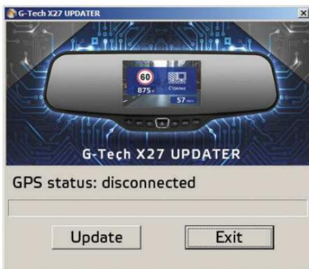
5. Connect the GPS module through the micro USB cable from the kit to the PC. If the connection is correct, the software will display «Connected» status
