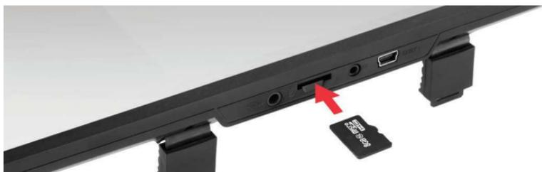
**CAUTION:** Attempting to insert a memory card with the wrong side may damage the device and the memory card itself. Make sure that the memory card is in the correct position.
