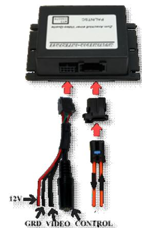
4. Connect the three Cinch sockets of the interface to the video source using a Video / Audio Cinch cable (not included). Reconnect the original Quadlock- connector to the COMAND.
