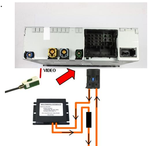
3. Connect the black wire of the cable kit to ground and the red wire to 12V plus. The corresponding control cable (e.g. for DVD device) is not supported.
