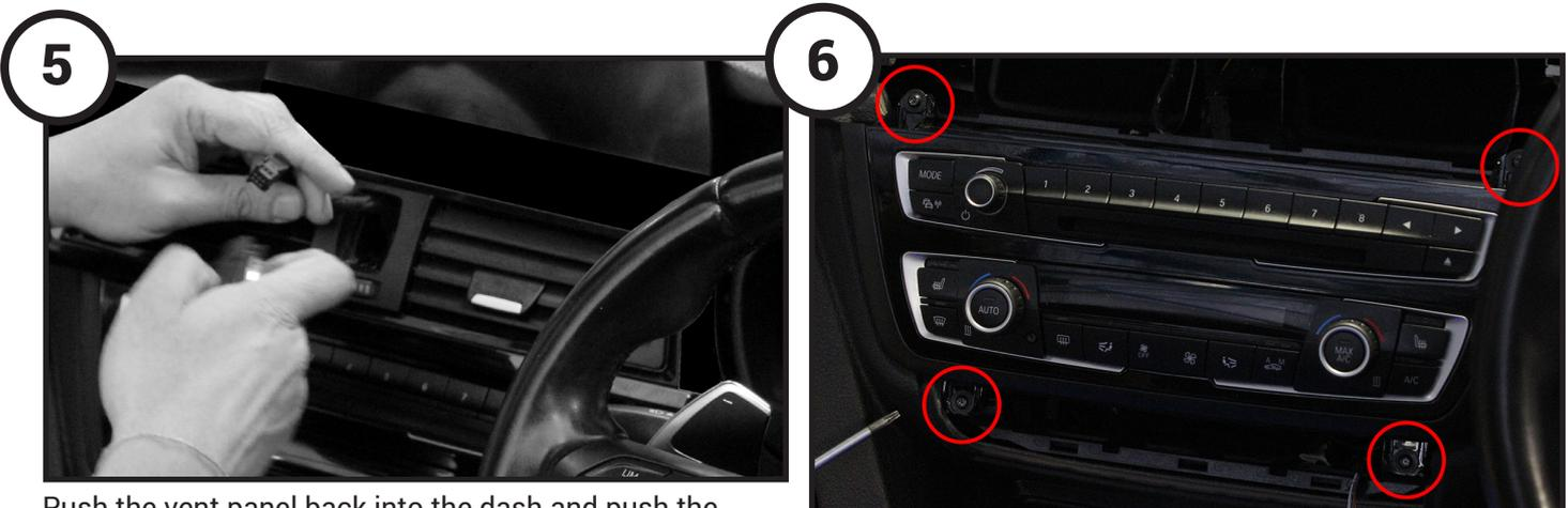
Push the vent panel back into the dash and push the hazard warning button out. Disconnect the button and fully remove the air vent panel/vents
