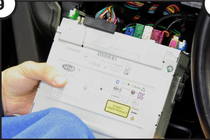
Remove the OEM head unit and disconnect all wiring to the unit. At this stage, the OEM head unit should be relocated into a suitable location at the rear of the vehicle.
