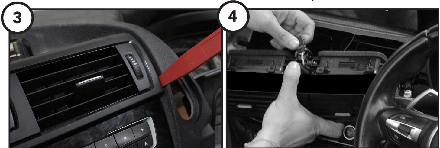
Use a panel removal tool to release the air vents and partially remove
