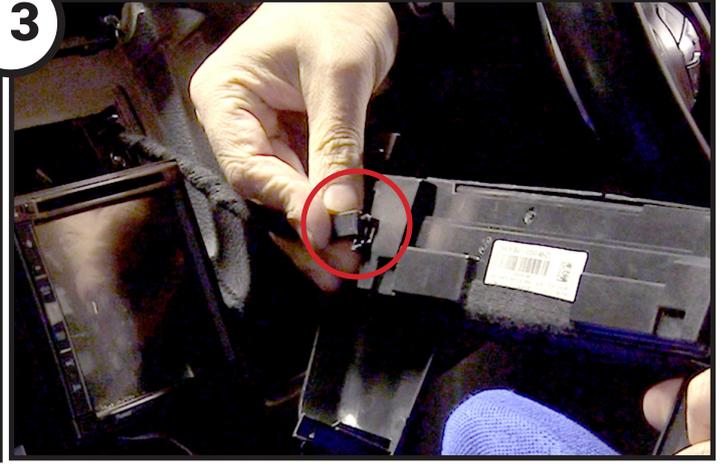
Reconnect the climate control button panel and attach the two clips included in the kit to the locations on the back of the double DIN fascia
