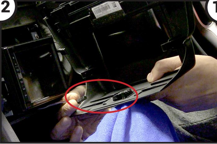
If the OEM panel has an LED located above the ashtray, remove this from the panel and slot it into the housing provided in the new panel to retain the ashtray light.
