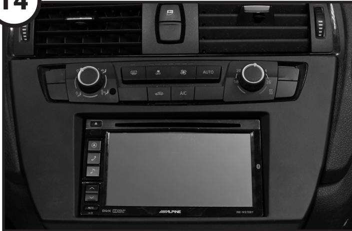
Fit the fascia into place around the stereo, using the clips to guide it into place. Screw into the dash using the OEM screws and locations. Reassemble dash in reverse order of disassembly to complete the installation.
