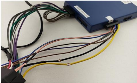
**STEP 2** Use spare wire to splice into the Yellow (B+) and Black (GND) wires in the vehicle-side harness.
