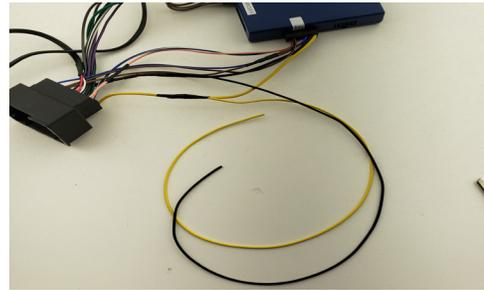
**STEP 3** Connect newly extended wires to the Yellow (B+) and Black (GND) wires on the radio-side harness as well as the Yellow (B+) and Black (GND) wires from the aftermarket radio.
