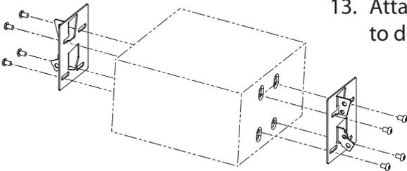
13. Attach mounting brackets to double DIN head unit
