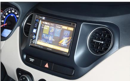
15. Mount air vents, OEM-clips and switch panel (with hazard light switch, passenger airbag switch etc.) to new fascia plate. Place fascia plate until it snaps in. Reinstall everything in reverse order to finish installation.
