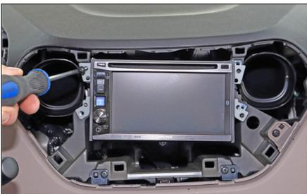
14. Connect all required circuit points. Place double DIN head unit on dashboard
