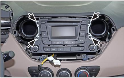
11. Remove 4 screws of OEM head unit
