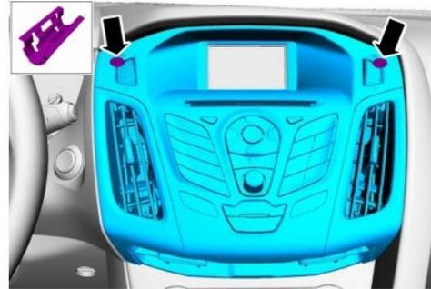
2. Carefully pop off the radio bezel making note that it is held by 2 clips as shown on the illustration above.
