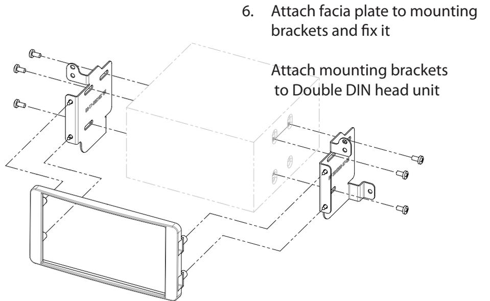
6. Attach fascia plate to mounting brackets and fix it
