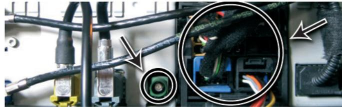
Disconnect the video cable from the Multimedia device (if available) and connect our video cable. The original must be connected to the VMX video-in socket. For further details, please check the hardware installation diagram. (Fig. 4)
