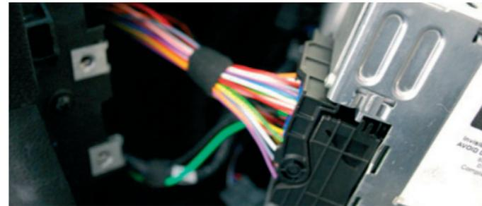
Remove the optical cable and the Quadlock connector. Follow the recommended installation on Fig 2., connect our Quadlock cable to the Head Unit and connect the original female Quadlock to the male end of our cable. For further details, please check Fig. 5.
