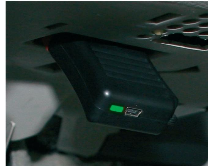
After the activation procedure turn your Audio System OFF (turn ignition OFF, remove the car key and close the doors) and wait approximately 2-3 minutes. After the required time period you can test the system functionality if the Gateway was already installed.
