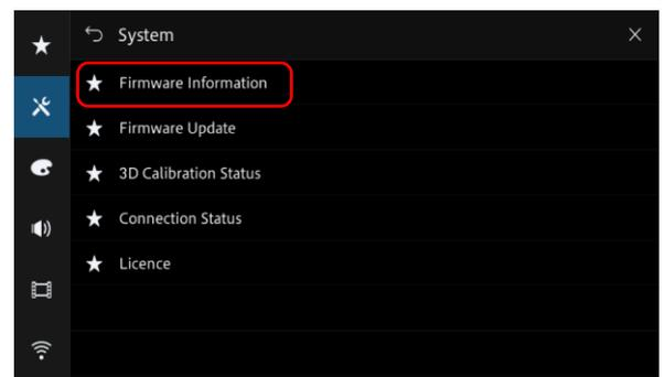
4. After the "Firmware Information" screen appears, check the firmware version; when the Version is lower than **3.00**, it is necessary to update the firmware.
